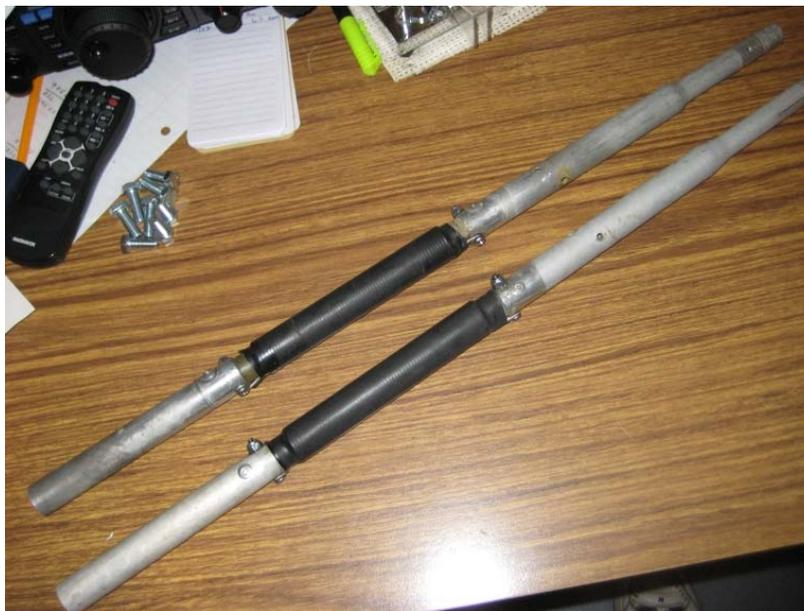
The final step was to tape up the ends of the coil using a first layer of 3M 130C covered by 3M 700 electrical tape. After replacing the broken aluminum boom and element tip, I'll be happy if the antenna only lasts another 15 years!
