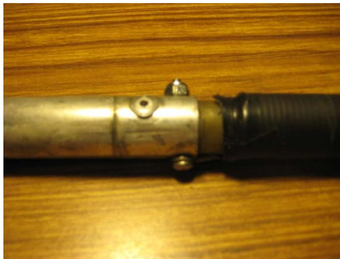
The aluminum extensions on the fiberglass coil form are pop riveted through the fiberglass. I found some of the pop rivets loose, allowing the end of the element to wiggle slightly, and to possibly cause the coil winding screw to loosen. I have seen and heard from others who had the same screws loosen on other antennas before, but never linked the possibility that it was because of loose pop rivets.
