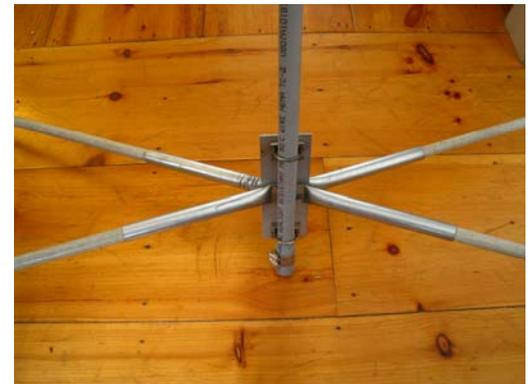
**Figure 5: TriMox hub and mast assembly**
