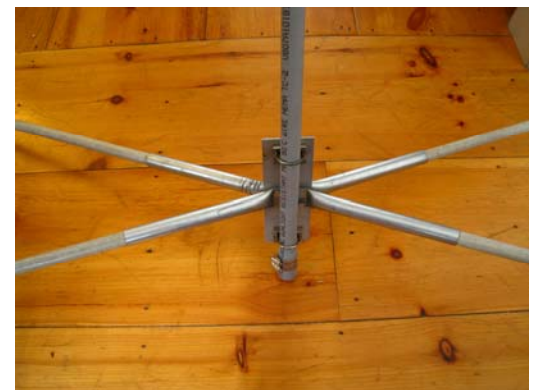
Figure 5: TriMox hub and mast assembly
