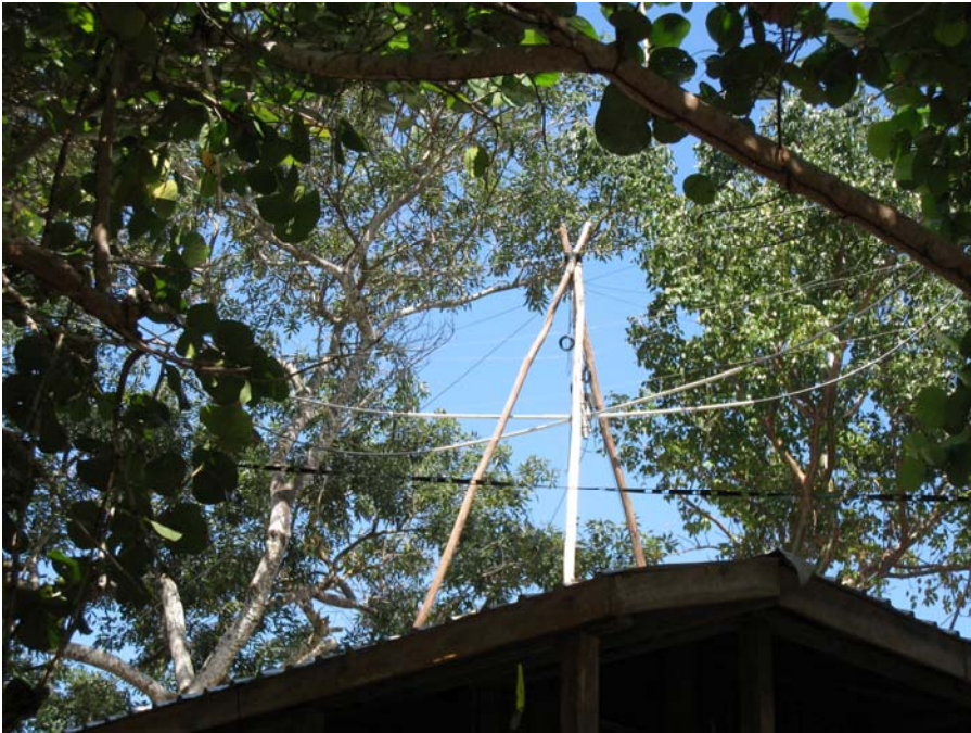
Figure 8: TriMox supported on cabana roof beneath makeshift wooden tripod
