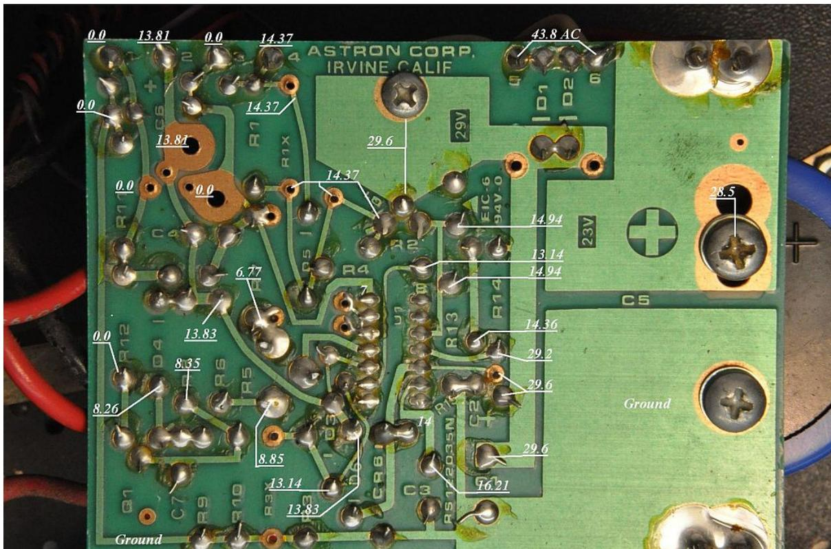
Should there still be a problem, the only component left to replace the LM723C. I suggest you replace it with an LM723 (no 'C'), as the 'C' designation indicates a commercial version, rated for 0 to 70 C, while the non-'C' version that is rated for -55 to +125 C.
