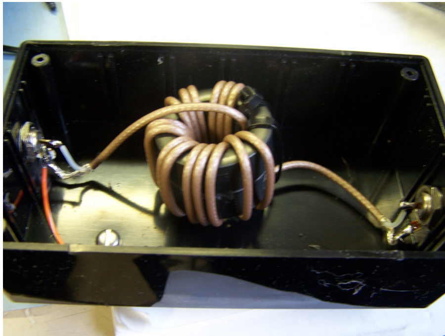
140-77 TOROID PAIR WITH 16 TURNS OF RG-179 AND AN ADDED GROUNDING LUG.
