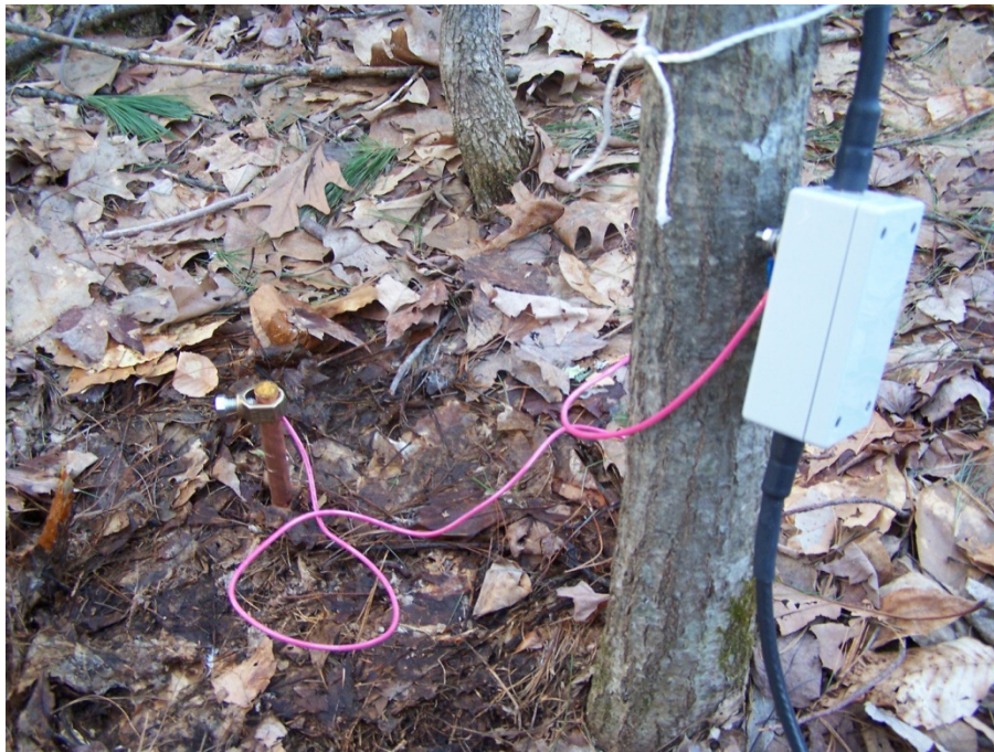
A COMPLETED COAX CHOKE IN PLACE OUT NEAR THE BEVERAGE TRANSFORMER. This was in a different box than I used in the later models.
