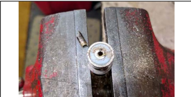
Photo 3: From a used PL-259, salvage a male tube to "fatten" the center conductor. It is, obviously, the proper size to go into the UHF barrel (double-female).
