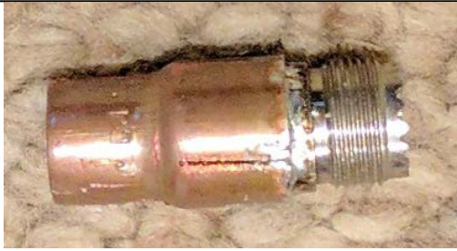
Photo 5: Solder barrel into copper “reducer” from hardware store. This step is “technique sensitive.” Too much heat and you will deform the plastic inside the barrel, making insertion of the PL-259 impossible, as the barrel will no longer line up with the threads for a straight insertion of the PL-259. The hacksaw slices make it easier to insert the barrel, and provide more surface area for solder to hold everything in place and make a good electrical connection. If you have removed the center barrel and its surrounding plastic, now is the time to re-insert and return the barrel to its original form and function, except for the fact that it is now soldered inside the reducer.
