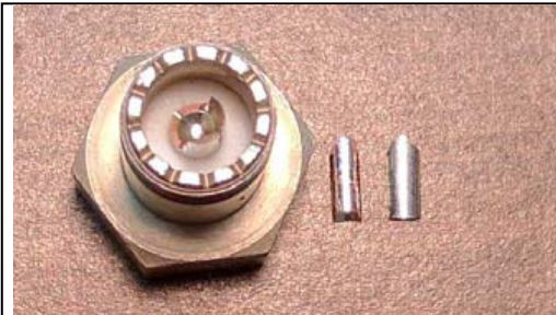
Photo 1: Broken fingers from the center conductor of my previous adapter. Almost every one of these I ever bought broke.
