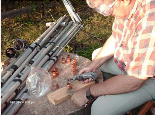
Photo 6: Add slits to the end of the reducer going over the hardline. I used a hacksaw.
