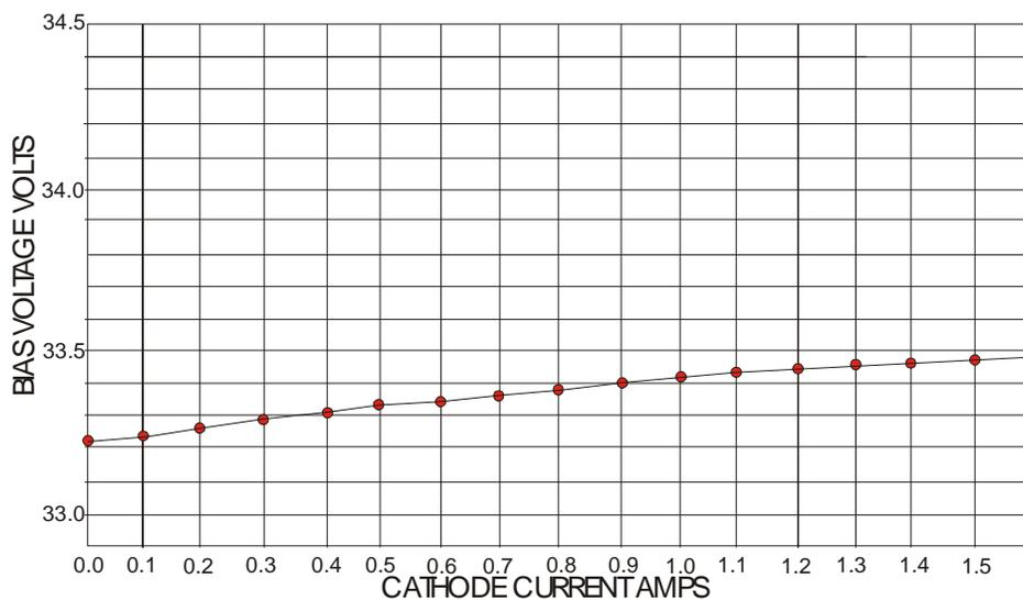
The TIP147 circuit seems to have a bit better shunt regulation performance than the MOSFET version. Impedance of the TIP147 design was about 0.2 ohms at 1 amp of current. Possibly the op amp gain in the MOSFET design could be adjusted for
