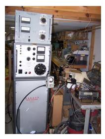
I tested the amplifier with a 0-5000 volt 1 ampere HV supply. You can see the K3 driver on the bench, and a wattmeter to measure power output. This is the power supply that I used to condition the old tube. The amplifier will do 1500 watts out with about 3600
