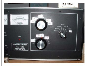
Another recent thread was about auto tune amps vs manual with marked dials. I mark my AL1500 with individual self adhesive labels, as shown in the photo. It's surprising how the settings hold over months on end.
