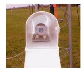
The mailbox-turned-capacitor cover has only been in use for a short time, but it has already endured some Michigan fall rains and kept the capacitor high and dry. The UVresistant plastic construction of the mailbox should provide many years of service.
