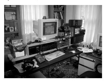
The photo shows the solution. Notice how the row of controls along the bottom of the FT-1000MP front panel are now easily accessible. Some people have asked if the main tuning knob is now too high. I have found that this new position provides easier operating of all controls!
