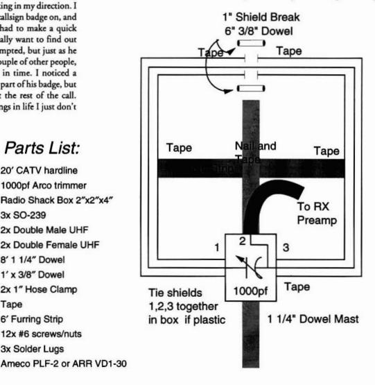
off the 1"of jacket required without breaking/weakening the center conductor of the hardline. When you are done, tape up the cut point and add some rigidity to the joint by placing some <sup>3</sup>/<sub>8</sub>" wooden dowel along and over the cutpoint and tape the whole joint again. When done, you will have a weatherproof joint and you will have restored the mechanical rigidity of the cutpoint as well.
