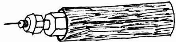
Figure 3: Slide heat shrink tubing over connector and clamp
