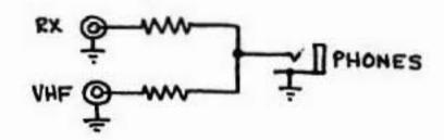
The resistors aren't critical - GQ uses 9 ohm/2 watt.
